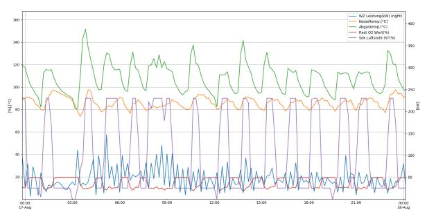
Figure 5. Various operating parameters of boiler 1 on a typical day in period 1
