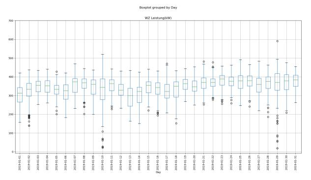
Figure 9. Snapshot of the load of the local heating network in January 2019. Circles: outlier, upper whisker: 1.5 \* IQR of box, box top: upper quartile, box middle: median, box bottom: lower quartile, lower whisker: 1.5 \* IQR of box#
