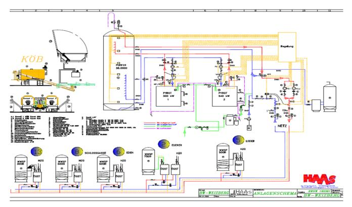
Figure 15. New hydraulic plan for storage implementation
