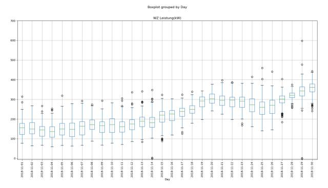
Figure 8. Snapshot of the the load of the local heating network in November 2018. Circles: outlier, upper whisker: 1.5 \* IQR of box, box top: upper quartile, box middle: median, box bottom: lower quartile, lower whisker: 1.5 \* IQR of box
