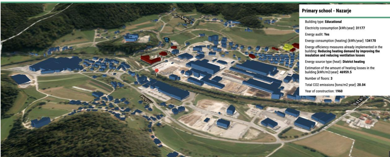
Figure 9: Generated 3D buildings in the PA6 Municipality of Nazarje, Slovenia
