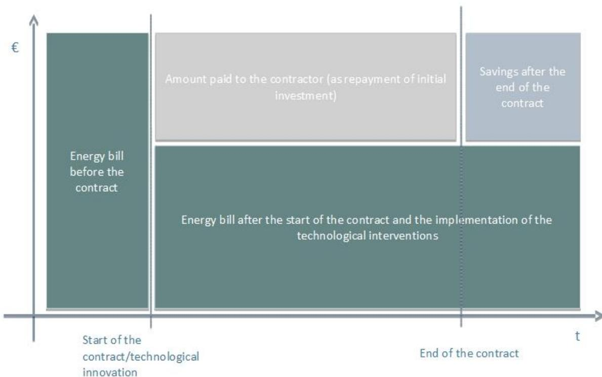
Figure 1: How a classic model of EPC works: advantages from the activation of an Energy Performance Contract for Public Administrations
