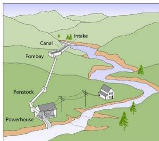
Figure 7.21: Type of Micro hybrid power plant; water is diverted into the penstock. Some generators can be placed directly into the stream, http://en.wikipedia.org/wiki/Micro_hydro#mediaviewer
