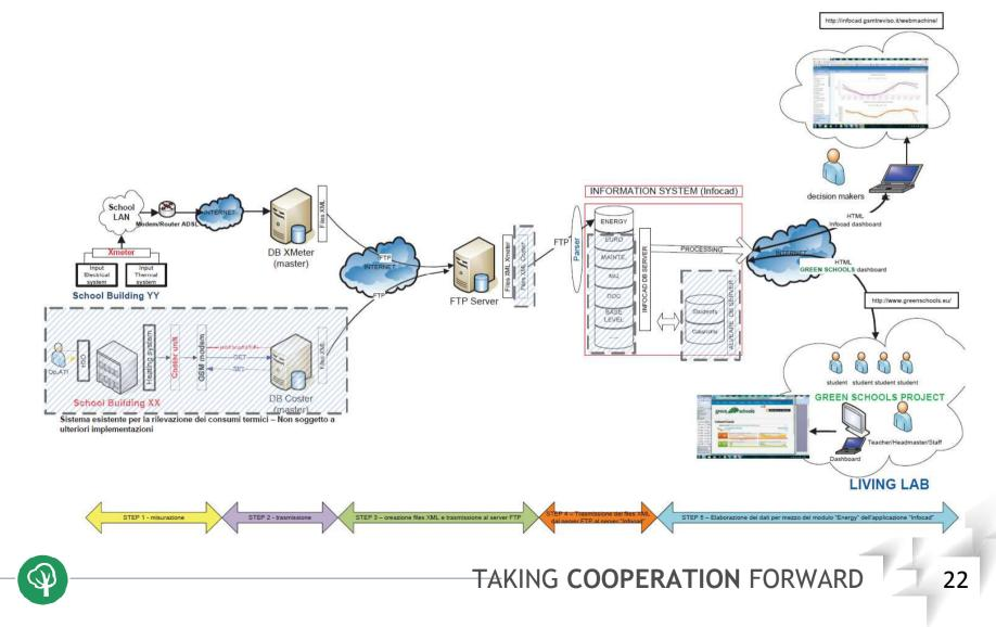
2. The monitoring system: retrieving/archiving flow of the data recorded by the SMART METERS
