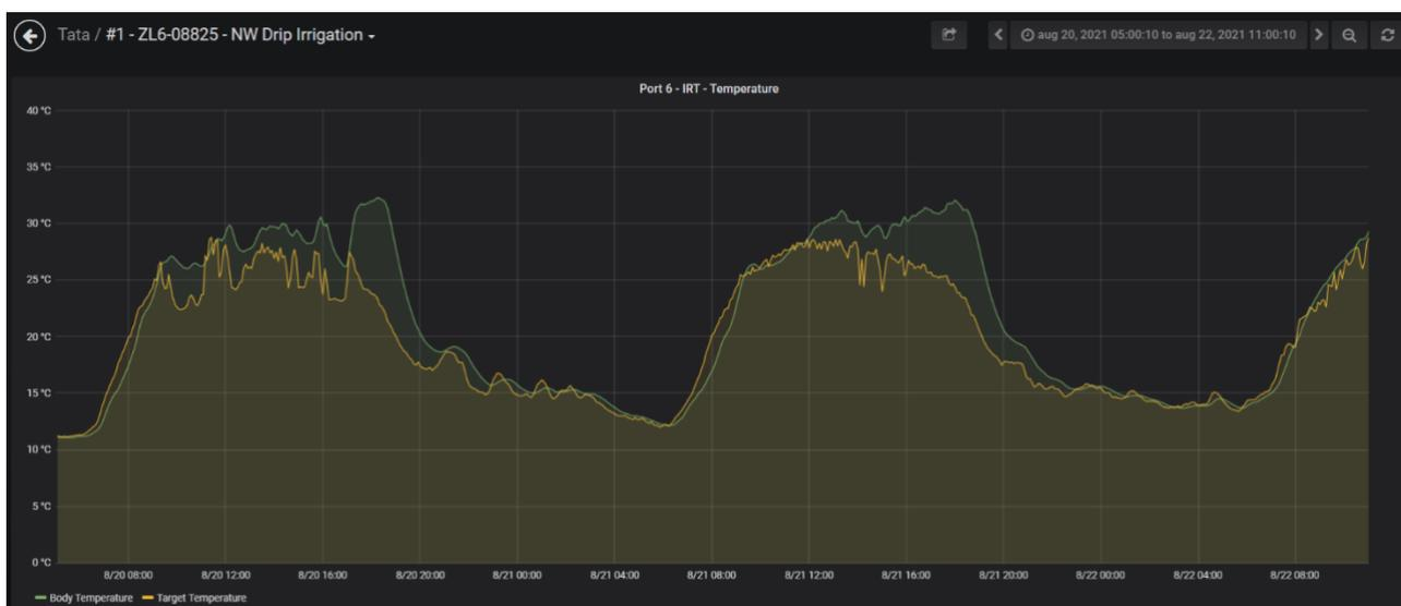
Figure 15: Canopy temperature (body and target) of the drip irrigated canopy on the SE side of the row from 20<sup>th</sup> August to 22<sup>nd</sup> August 2021.
