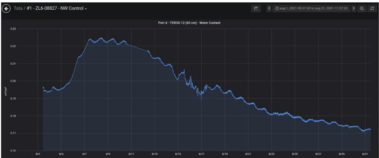
Figure 11: Soil water content at 60 cm in the rainfed row from 1<sup>st</sup> August to 31<sup>st</sup> August 2021.
