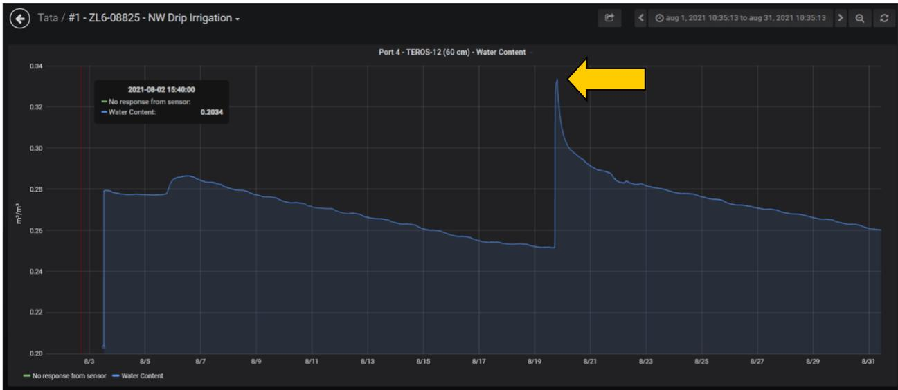
Figure 10: Soil water content at 60 cm in the drip-irrigated row on the NW side of the canopy from 1<sup>st</sup> August to 31<sup>st</sup> August 2021. (arrow indicates the date of the irrigation)
