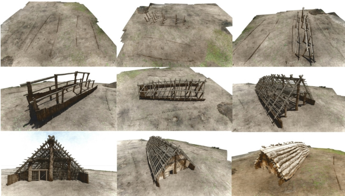
Fig. 13: Phasing of one of the possibilities of construction of a long Neolithic house visualized on a 3D SfM model (images: J. Unger, ARUP).
