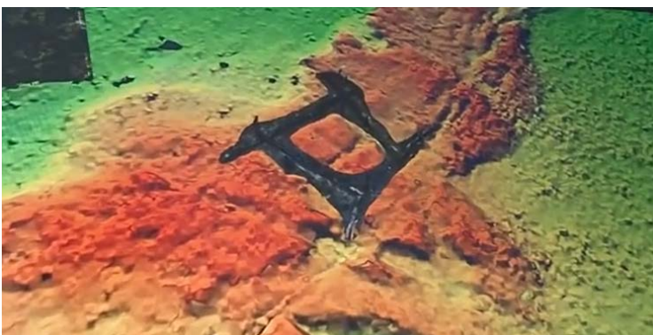
Fig 16: Implementation of photogrammetric model into hydroacoustic image (UMK)
