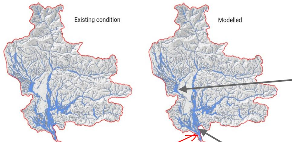
Figure 10: Graphical representation of calculated flooding for 15 hours event with 100year return period. Existing conditions flooding is on the left side, flooding with implemented proposed NSWRM (dams) is on the right. On first look, difference is negligible.
