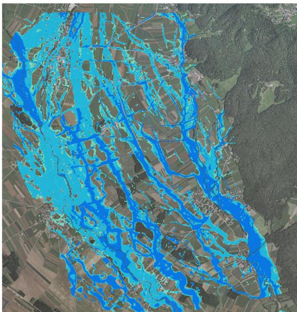
Flood routing with retentions on the alluvial fan (Cerklje na Gorenjskem)
