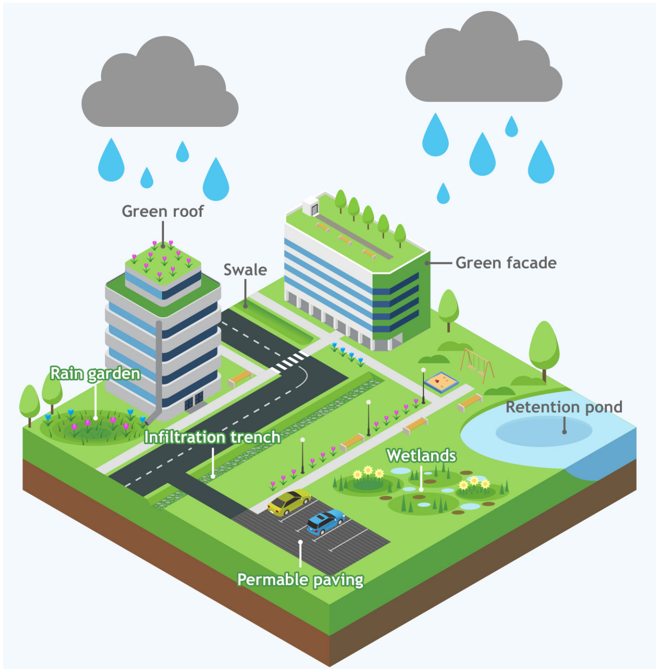
Figure 3: Rainwater management tools.
