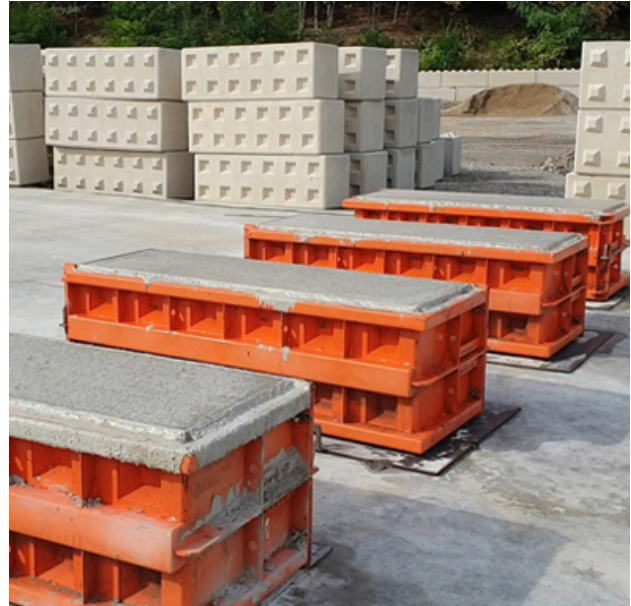
Produced concrete blocks (CWC and Cinderella projects). Photo: Aleš Erker, MBVOD.
